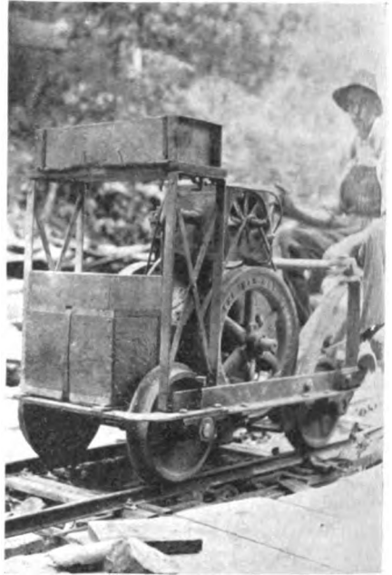
HOME-MADE TRACTION ENGINE FOR HAULING CEMENT AND CONCRETE THROUGH THE TUNNEL LINE
